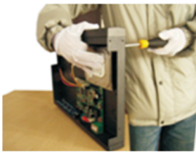
1.Install fixed screw for HDD
